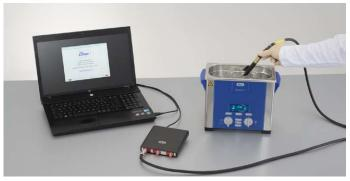
Elmasonic P 30 H during the cavimeter test
