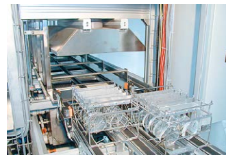
Intermediate cleaning of precision optics and ready-for-coating cleaning systems.
